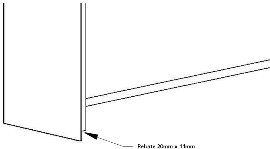
2. Fix the plinth to the floor and wall using the brackets supplied, ensuring that the top of the plinth is level (if multiple Hygipods are being installed, continuous plinth may be supplied, to be cut to length on site).
