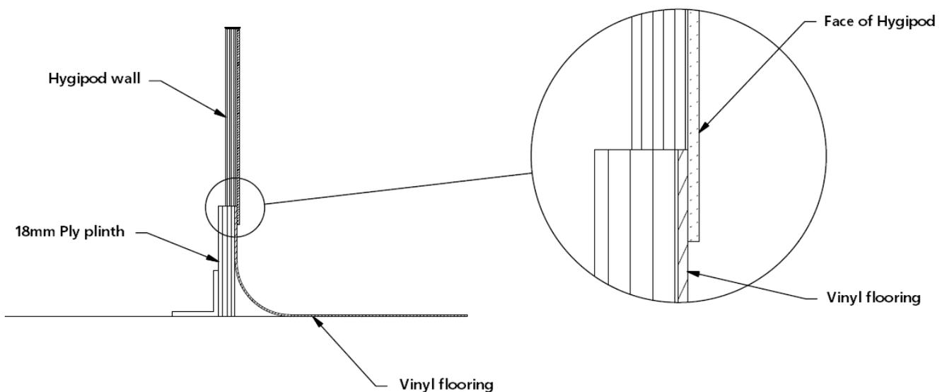
3. If vinyl flooring is to be covered to the plinth, this should be installed at this stage.
