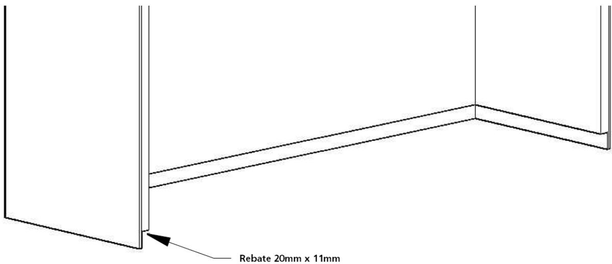
2. Fix the plinth to the floor and wall using the brackets supplied, ensuring that the top of the plinth is level (if multiple Hygipods are being installed, continuous plinth may be supplied, to be cut to length on site).
