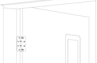
10. Remove the bracing from the top corner and across the bottom of the frame.
