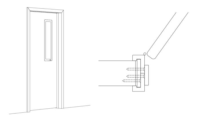
13. Peel back any protective film from the area covered by the doorstop, and fit the ply/MDF doorstop head, using 45mm screws (supplied) leaving a 2mm gap between the doorstop and the door leaf for the PVC doorstop cover.
